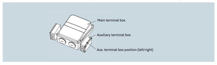
Motors of frame sizes 225S to 355L are available with up to 4off auxiliary Terminal Boxes. The position of the cable entries to the auxiliary Terminal Boxes should be advised at the order placement.
